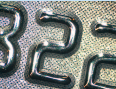
Steep incident light with the 3 upper diodes
